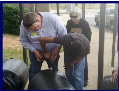
Student drills hole for bushing and spigot with guidance by Mr. Oxner.
