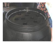
3. Drill a hole (with a 1¾" hole saw) at the top of the barrel for an overflow and one at the bottom of the barrel for the spigot. If barrel will not be elevated locate hole for spigot high enough to attach hose without crimping.
